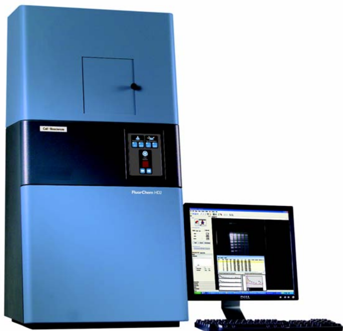
Figure 1-2: Multimage II Light Cabinet (DE-500)—Pictured with the cabinet top (DE-500FC)
